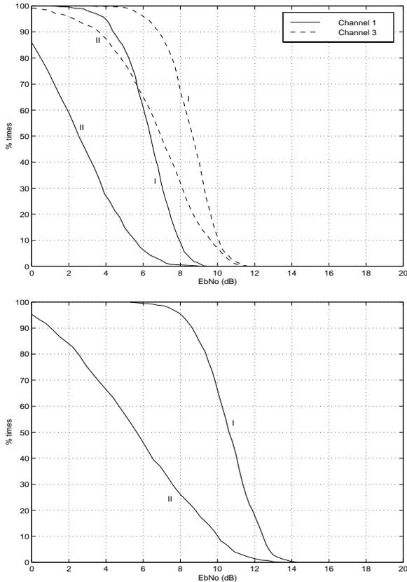
Figure 2. Algorithm performance in temporal diversity (upper plot) and spatial diversity (lower plot) for an  $E_bN_0=12$ dB. Comparison of the algorithm with (I) and without (II) the use of linear block codes.
