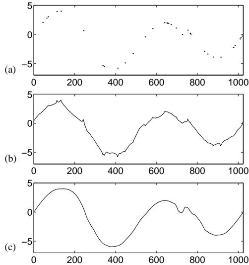
Figure 3: *Maximum-smoothness interpolation of 32 nonuniform samples of the HeaviSine signal. (a) 32 nonuniform samples. Maximum-smoothness interpolation with (b)  $\alpha = 0.8$  and (c)  $\alpha = 2.0$ .*
