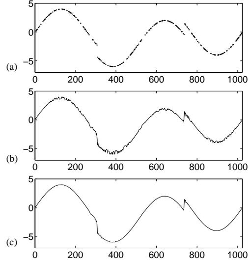
Figure 2: Maximum-smoothness interpolation of 256 nonuniform samples of the HeaviSine signal. (a) 256 nonuniform samples. Maximum-smoothness interpolation with (b)  $\alpha = 0.5$  and (c)  $\alpha = 0.9$ .
