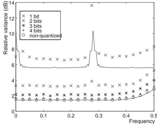
Figure 3: Variance versus frequency for  $N = 32$  and  $\text{SNR}=12$  dB for 4-th order Butterworth filters (see, table 1 in [2]). The number of ensembles for each frequency was 10000 with random phase.
