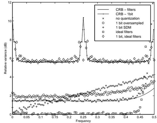
Figure 4: Variance versus frequency for  $N = 32$  and  $\text{SNR}=12$  dB for 4-th order Butterworth filters (see, table 1 in [2]). The number of ensembles for each frequency was 10000 with random phase.
