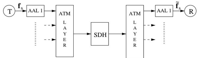
Figure 1: Transmission network:  $T$  transmitter,  $R$  receiver
