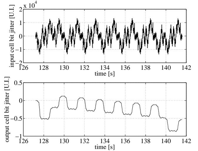
Figure 5: Input and output jitter at steady state.
