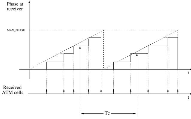
Figure 2: Ideal phase module  $\text{max\_phase}$  (dashed line) and real phase module  $\text{max\_phase}$  (solid line) at receiver.
