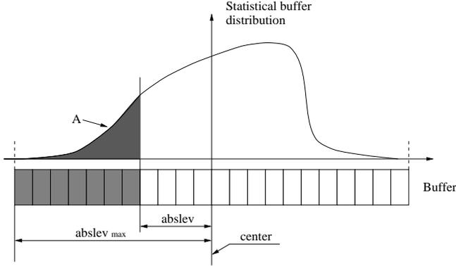
Figure 4: Definition of buffer parameters related to a generic distribution.
