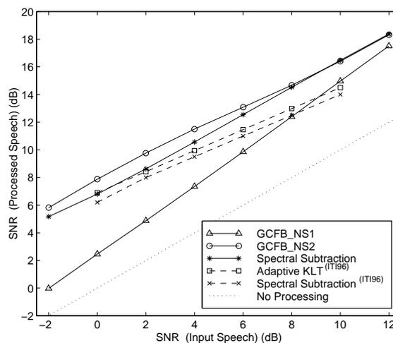
**Figure 4.** Performance comparison between Gammachirp Filterbank Noise Suppression (GCFB\_NS) and Spectral Subtraction (solid lines). The results represented by the dashed lines (IT196) are adapted from [11].
