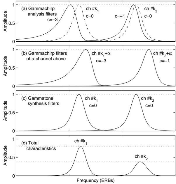
**Figure 2.** Schematic graphs for explaining the principle of noise suppression. Amplitude spectra of gammachirp and gammatone filters are plotted as a function of frequency (arbitrary ERB rates). See text for more detail.
