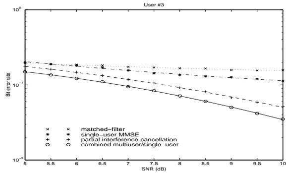
**Figure 3.** Bit error rate vs. SNR for four receivers in the presence of unknown interferers.
