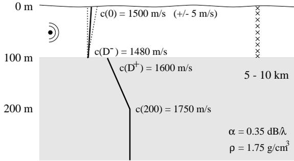
Figure 4: Range independent shallow water ocean model.
