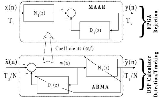
Figure 2-3: Main Structure of the PIRANHA Cell  $H_1(z)$ .
