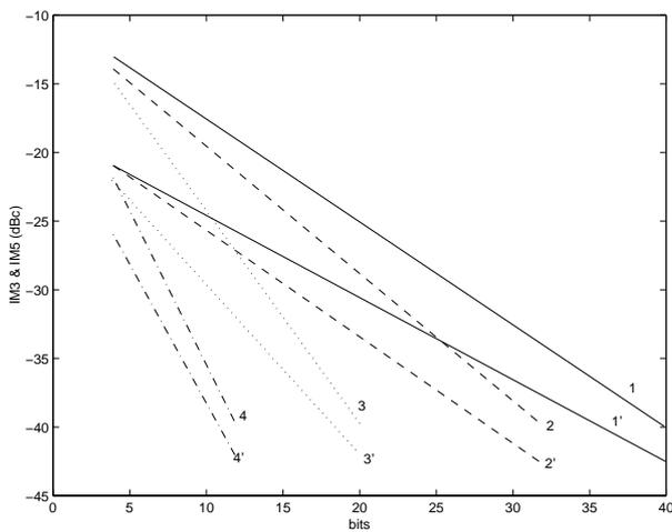
Figure 10: Temporal evolution of the 3<sup>rd</sup> and 5<sup>th</sup> order intermodulation products. Lines 1 and 1': system with [BO]=10 dB. Lines 2 and 2': [BO]=4 dB. Lines 4 and 4': [BO]= 10 dB.
