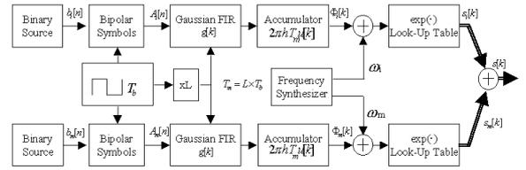
Figure 7: Architecture of the Multicarrier predistorter. Baseband combination of CPM carriers.
