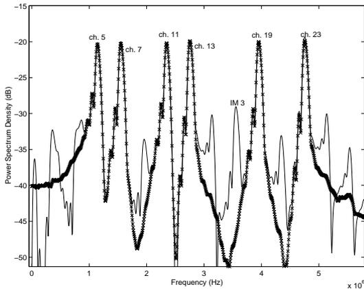
Figure 9: PSD with  $N=6$ . Continuous line: no predistortion. Symbol X: with predistortion.
