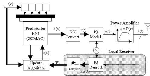
Figure 8: Architecture of the Multicarrier predistorter. Predistorter.
