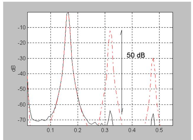
Figure 6: Harmonics in amplification with and without predistortion. The amplifier saturated.
