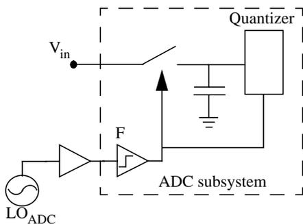
Figure 5. Receiver sampling stage.
