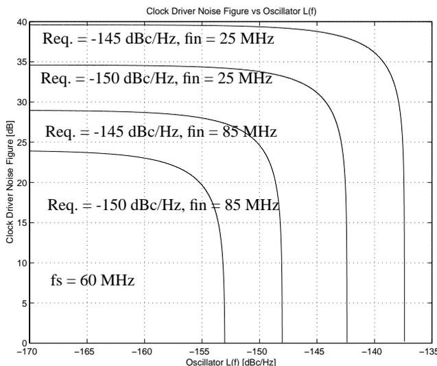
Figure 6. Required combination of LO phase noise and clock drive amplifier noise figure.
