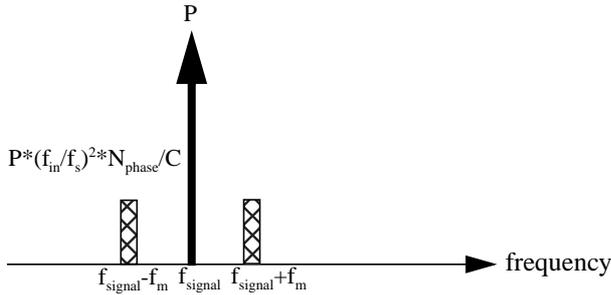
Figure 2. Noise sidebands of the sampled signal. Levels are average power.
