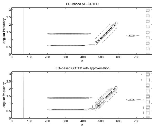
Figure 2: On the top is the AF-GDTFD computed using the first six largest eigenvalues and standard FFT. Below is the result if the additional approximation is performed using the proposed approach.
