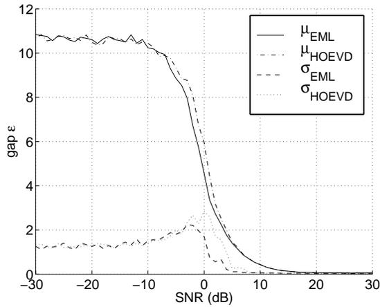
Figure 1: Mean ( $\mu$ ) and standard deviation ( $\sigma$ ) of gap  $\varepsilon$  for a mixture of 3 uniformly distributed sources in additive Gaussian noise.
