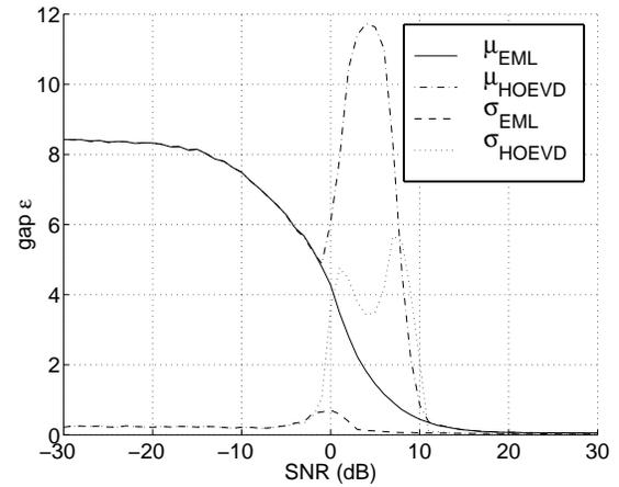
Figure 2: Mean ( $\mu$ ) and standard deviation ( $\sigma$ ) of gap  $\varepsilon$  for a mixture of 3 uniformly distributed sources in additive uniform noise.
