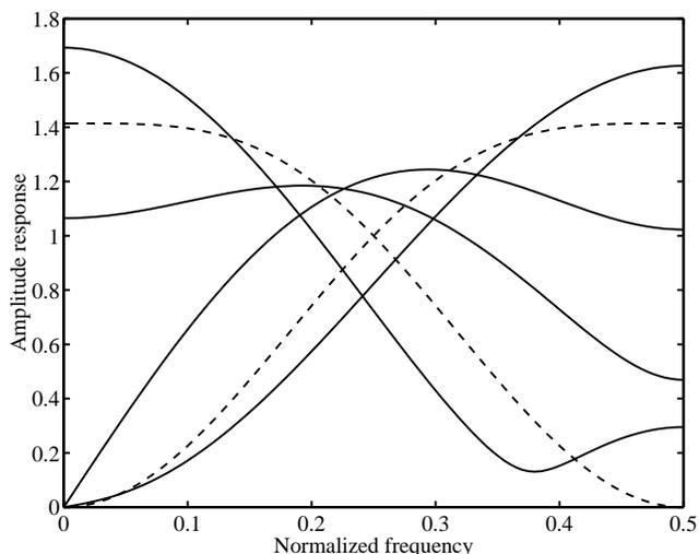
Figure 3: Length-3 boundary filters (solid lines) without DC leakage based on minimum-phase length-4 Daubechies filters (dashed lines).
