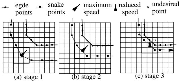
Figure 1. Movement of the snakes with  $E_{\text{feedback}}$ .
