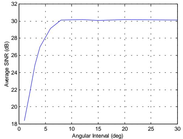
Fig.2 Performance of signal separation based on estimated array response.
