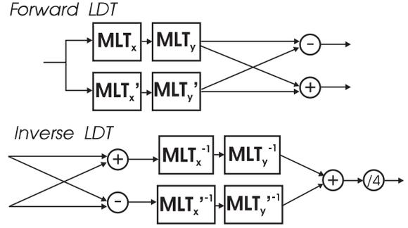
Figure 1: Block diagram of the LDT and its inverse.
