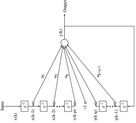
Figure 1: NARMA(p,q) recurrent perceptron
