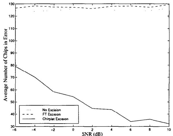
Figure 2: Average number of chips in error per information bit as a function of SNR. SIR =  $-26$  dB, and chirp-rate of 0.5 are selected.
