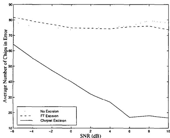
Figure 4: Average number of chips in error per information bit as a function of SNR.  $\text{SIR} = -2$  dB, and chirp-rate of 0.5 are selected.
