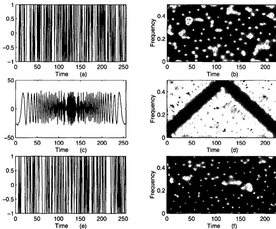
Figure 3: Chirp interference excision example for  $\text{SNR} = -6$  dB,  $\text{SIR} = -26$  dB, and chirp-rate = 0.5. (a) The PN sequence, (b) STFT of the PN sequence, (c) received signal that consists of the PN sequence, jammer, and white Gaussian noise, (d) STFT of the received signal, (e) interference excised and binary quantized signal, (f) STFT of the interference excised signal.
