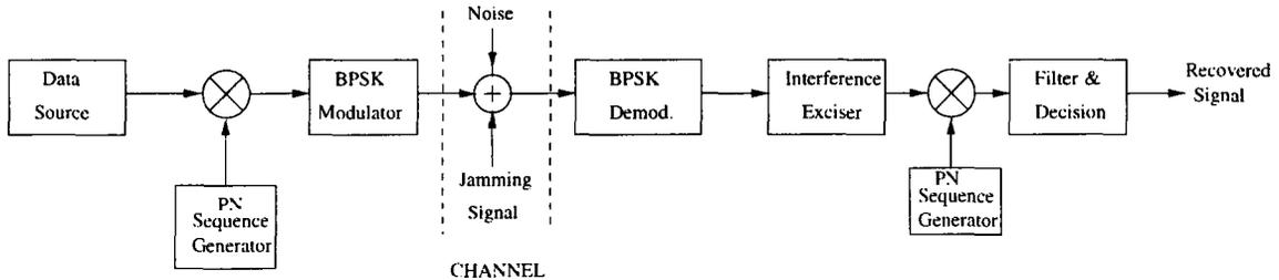
Figure 1: Block diagram of a DSSS communication system [1].
