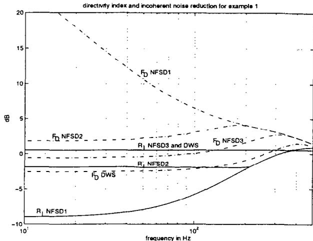
The comparison of the delay-weight-sum (DWS) beamformer with the NFSD algorithm shows several surprising results (figure above, note that  $f_{\text{aliasing}} = 340 / 0.6\text{Hz} = 567\text{Hz}$ ) :
