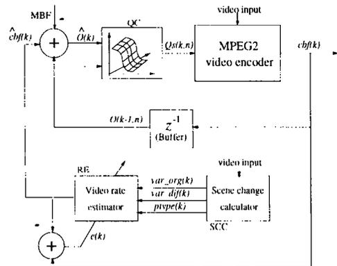
Figure 3. The structure of the feed-forward network for MPEG rate control.
