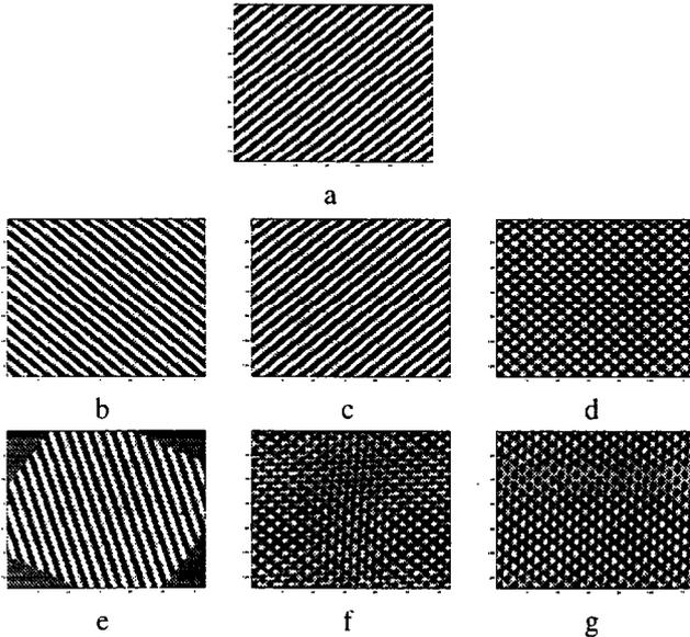
Figure 1: Measuring the distance between synthetic textures using Kullback's distance measure. In decreasing order : a) Texture H1 – the reference texture; b) Texture H1, 90 degree rotated, c) Texture H1, translated d) Texture H2, e) Texture H1 .60 degree rotated, f) Texture H4, g) Texture H3
