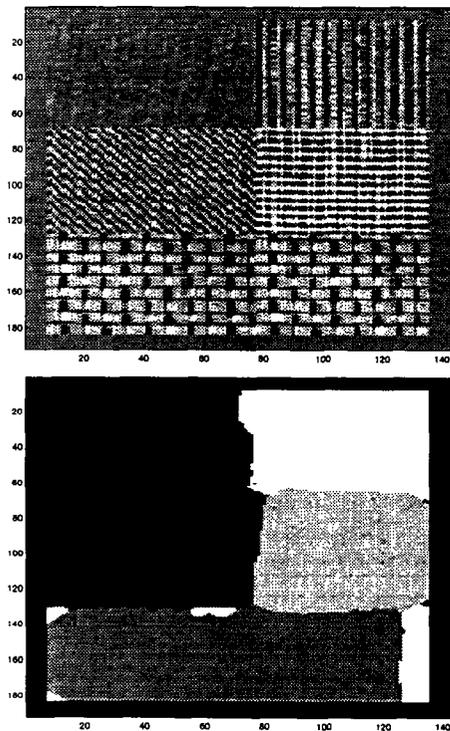
Figure 3: Unsupervised segmentation of Brodatz textures: Original image (top); Final segmentation, after 100 iterations (bottom).
