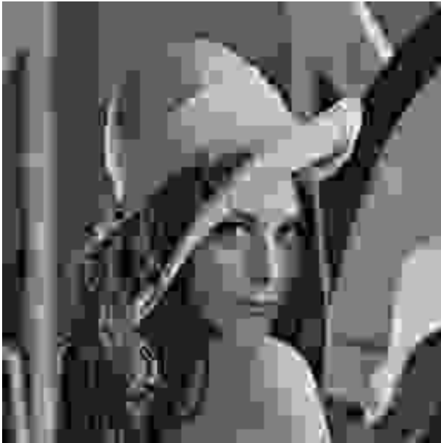
Figure 5: JPEG ( R=0.20\text{bpp} , \text{PSNR}=23.19\text{ dB} )
