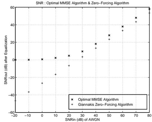
Figure 3:  $SNR_{out}$  performance of the proposed optimal MMSE based equalizer and zero-forcing equalizer used in [5] vs  $SNR_{in}$ . For (5,9) case of transmission channel given in [3].
