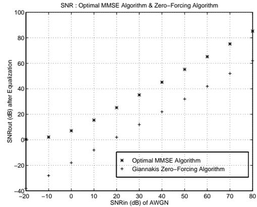
Figure 4:  $SNR_{out}$  performance of the proposed optimal MMSE based equalizer and zero-forcing equalizer used in [5] vs  $SNR_{in}$ . For (8,15) case of transmission channel given in [5].
