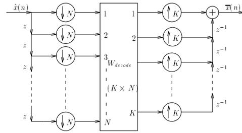
Figure 2: The proposed Nonmaximally Decimated Filterbank Based Decoder / Post-equalizer structure for Blind Channel Identification and Equalization.
