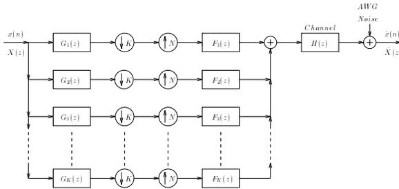
Figure 1: The proposed Nonmaximally Decimated Filterbank Based Precoder / Pre-equalizer structure for Blind Channel Identification and Equalization.
