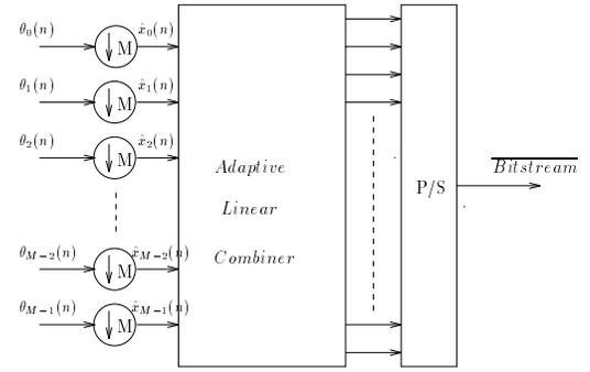
Figure 7: Adaptive linear combiner after the analysis filter bank at the receiver of DSBMT.
