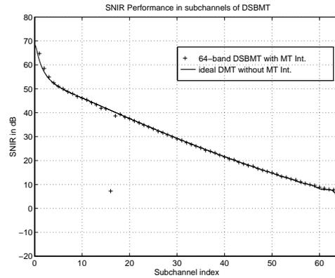
Figure 8: DWMT (DSBMT) Multicarrier Transceiver Performance in Multitone Interference Environment on AWG 26 9kft loop plant.
