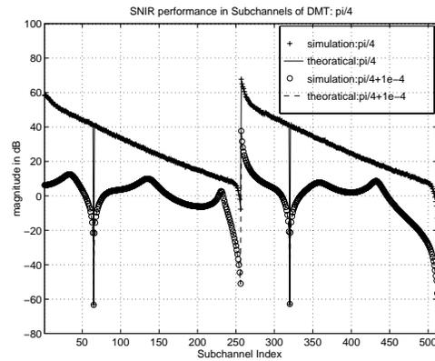
Figure 3: The sensitivity of SNIR for each subchannel of DMT based system for a single-tone interference and AWGN scenario with  $\omega_{st} = \frac{\pi}{4}$  and  $\omega_{st} = \frac{\pi}{4} + 0.0001$  on AWG 26, 9 Kft loop plant, *SNIR* = 0dB .
