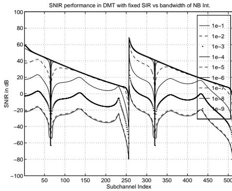
Figure 5: The performance of SNIR in each subchannels of DMT based system in different NB bandwidth with fixed SIR and center frequency  $\omega_{sto} = \frac{\pi}{4}$ .
