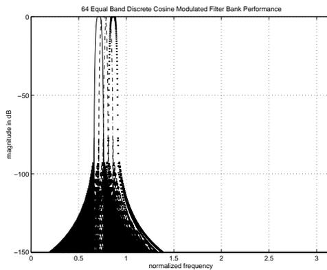
Figure 6: Frequency Response of Subcarrier 15, 16, 17 and 18 of a 64 Equal Band Discrete Cosine Modulated Filter Bank.
