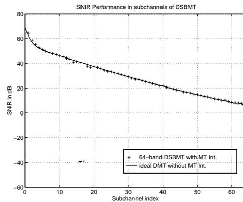
Figure 9: DWMT (DSBMT) Multicarrier Transceiver Performance in Multitone Interference Environment on AWG 26 9kft loop plant.
