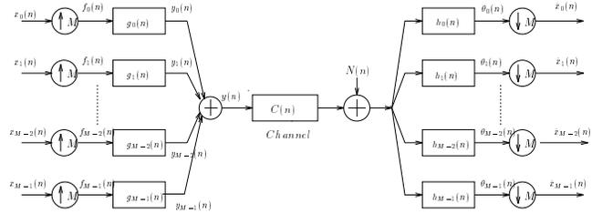
Figure 1: Basic Structure of a Multicarrier based digital transceiver.
