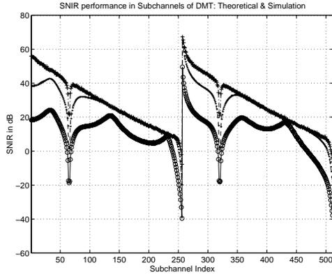
Figure 4: The theoretical and simulation SNIR performance of each subchannels of DMT based system with fixed center frequency  $\omega_{sto} = \frac{\pi}{4}$ , NB bandwidth is  $0.01\pi$ ,  $SIR = 40dB$ ,  $SIR = 60dB$ , and  $SIR = 80dB$ , respectively.
