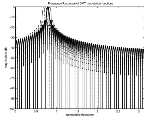
Figure 2: Frequency Response of Subcarrier 15, 16, 17 and 18 of 128 point DFT basis functions.
