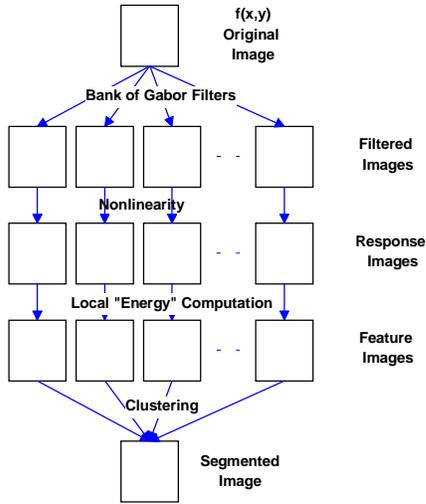
Fig. 2: An overview of the texture segmentation algorithm
