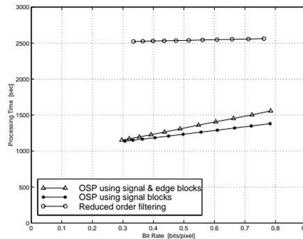
(b) Bit-rate vs processing time.
