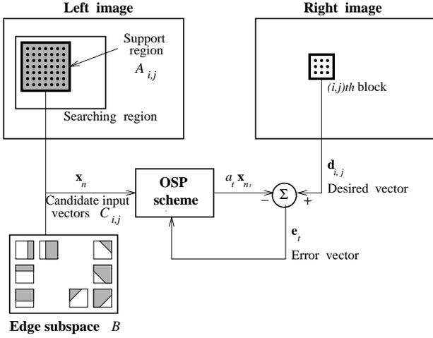
Figure 1: The orthogonal subspace projection (OSP) scheme for stereo image compression.
