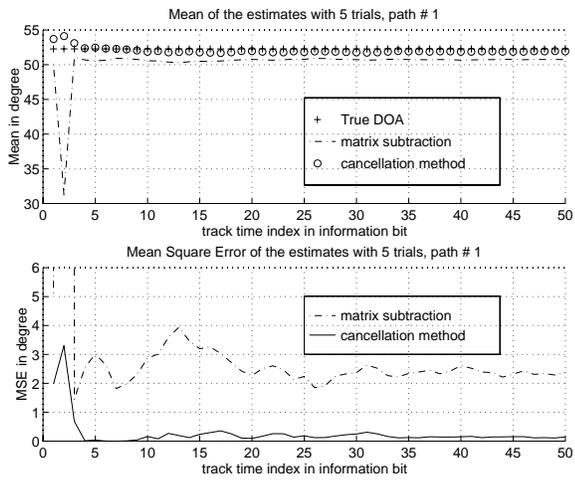
Figure 1: DOA of path 1 for 5 antenna elements and 25 mobiles each with 3 multipaths
