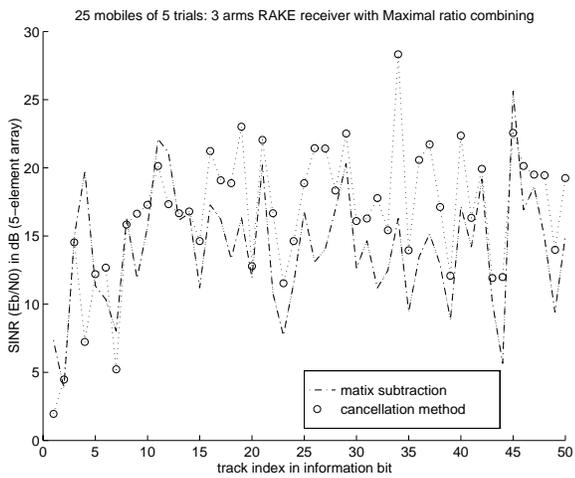
Figure 2: Output SINR for 5 antenna elements and 25 mobiles each with 3 multipaths
