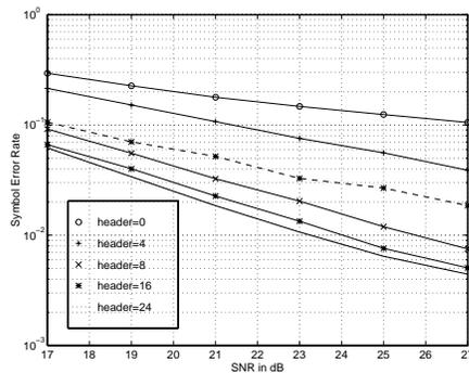
Figure 4: Symbol Error Rate vs. SNR. Solid lines: Using blind channel estimation. Dashed lines: Using non-blind channel estimation.
