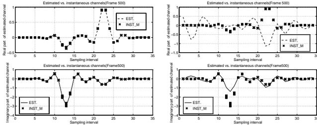
Figure 3: Instantaneous channel vs. estimated channel for header length 8 (left: blind channel estimation, right: header-aided non-blind channel estimation)
