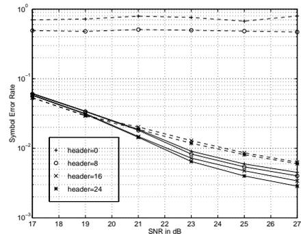
Figure 2: Symbol Error Rate vs. SNR. Solid lines:Using blind channel estimation. Dashed lines: Using header-aided channel estimation.
