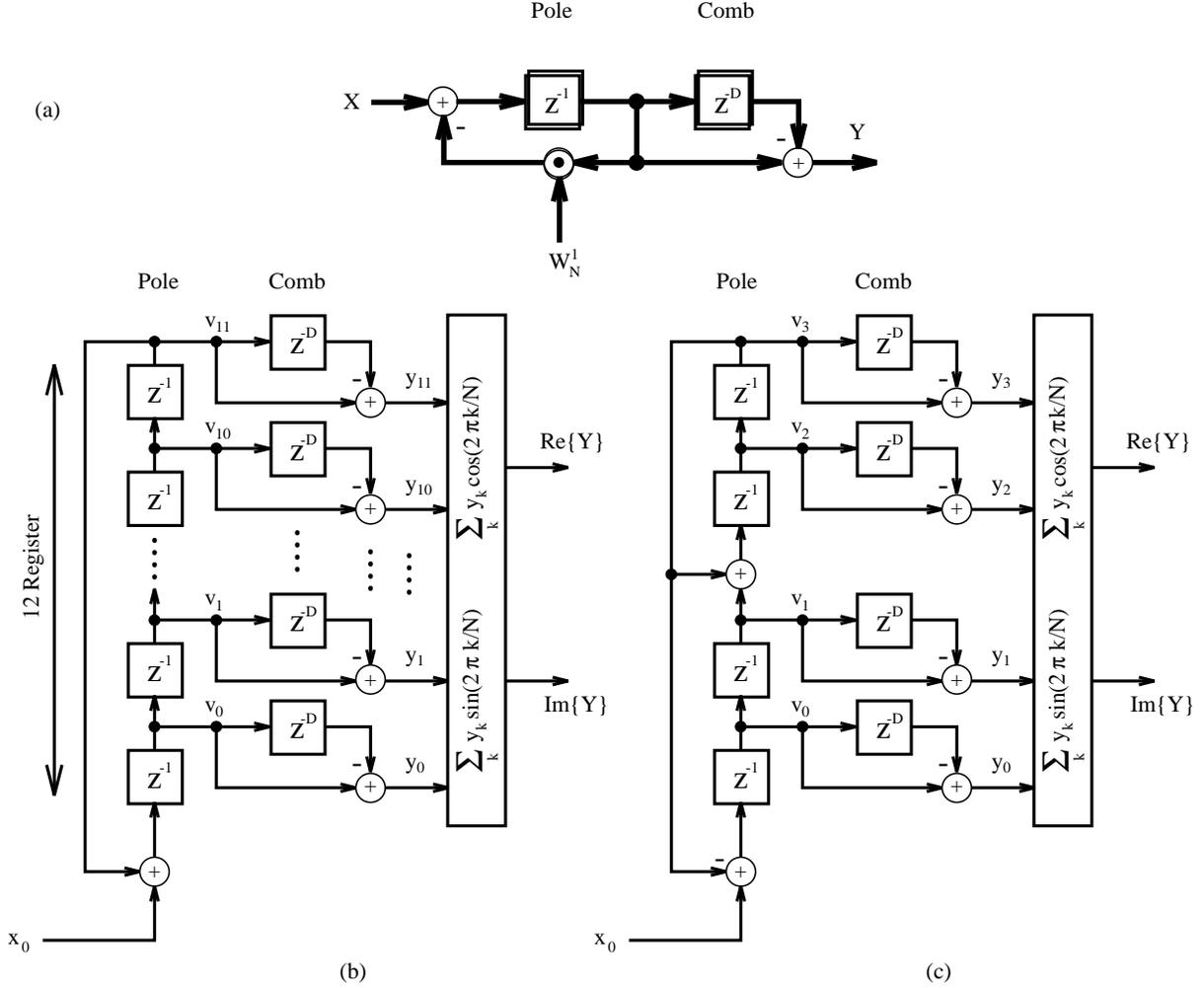
Figure 2: One stage FSF for  $N = 12$  and pole at  $W_{12}^1$ . (a) One pole FSF filter (shadowing symbolizes the processing in parallel channels for algebraic integers). (b) Without cyclotomic polynomial reduction. (c) Using the cyclotomic polynomial  $C_{12}(x)$ .
