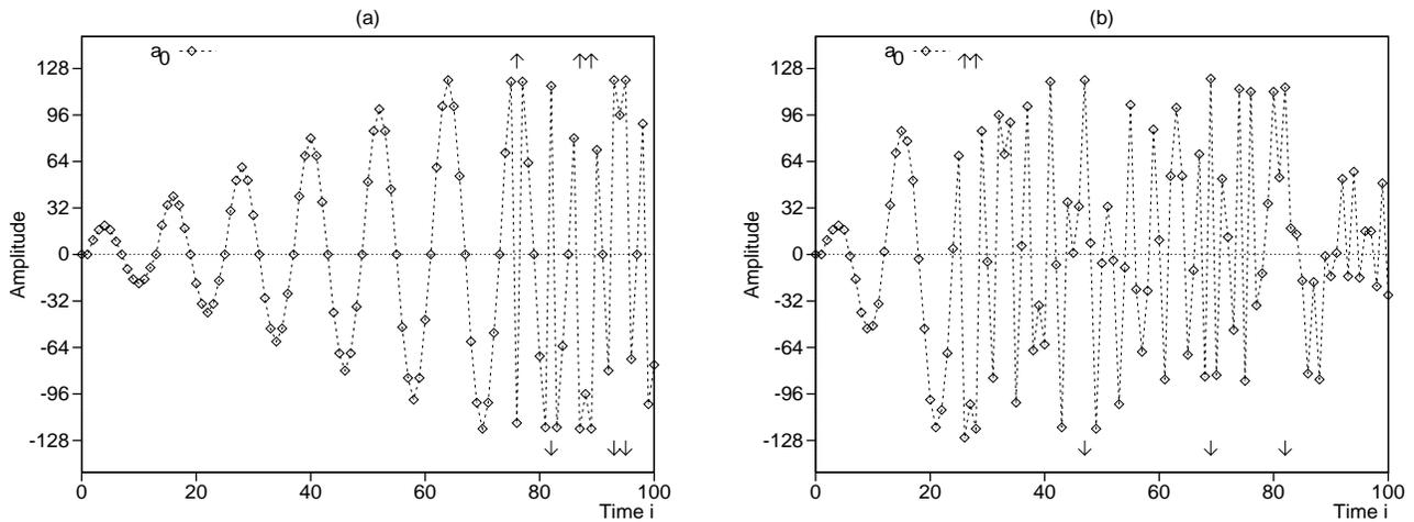
Figure 4: Overflow behavior to Figure 3 for  $v_0$  with eigenfrequency test  $D = 12$ . Modulus is 256. (a) Pole without modulo reduction. (b) Pole with modulo reduction.
