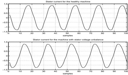
Figure 3: stator current data for the healthy and the damaged machine
