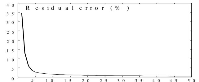
**Figure 5.** Residual relative error as a function of iterations number
