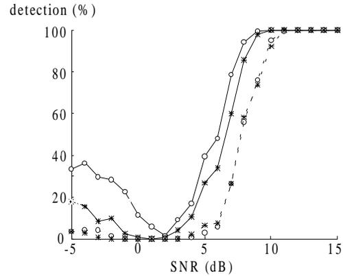
Fig. 6. Probability of detection with Gaussian nonwhite noise and  $A_1 = A_2$  from -5 dB to +15 dB.
