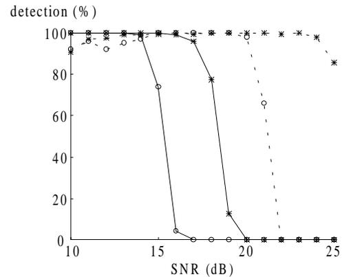
Fig. 7. Probability of detection with Gaussian nonwhite noise ( $A_1 = 10$  dB,  $A_2$  varies from 10 dB to 25 dB on the x-axis).
