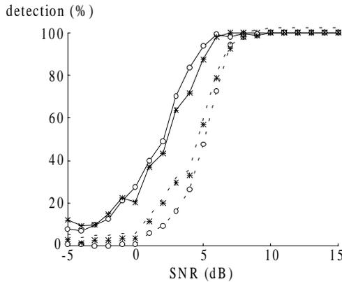
Fig. 4. Probability of detection with Gaussian white noise and  $A_1 = A_2$  from -5 dB to +15 dB.
