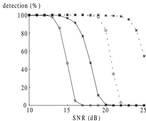
Fig. 5. Probability of detection with Gaussian white noise ( $A_1 = 10$  dB,  $A_2$  varies from 10 dB to 25 dB on the x-axis).
