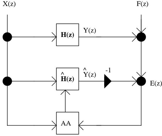
**Figure 1.** Signal-flow graph representation: AA-adaptive algorithm;  $H(z)$ -echo path transfer function;  $\hat{H}(z)$ -adaptive filter transfer function.
