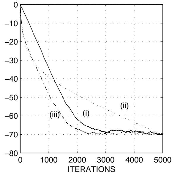
**Figure 4.** Normalised tap-error vector norm, dBs versus the number of iterations in the case of LMS (i), LMF (ii) and CFA(iii) with 20 averages.
