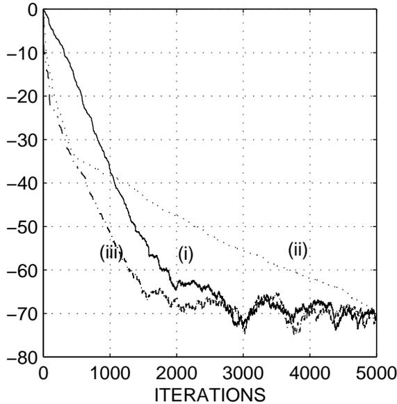
**Figure 3.** Normalised tap-error vector norm, dBs versus the number of iterations in the case of LMS (i), LMF (ii) and CFA(iii) with no average.
