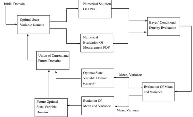
**Figure 3. The Block Diagram of the Optimal State Variable Domain Determination**
