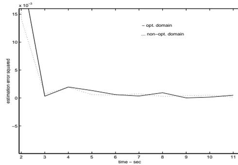
**Figure 4. The estimation accuracy with and without optimal truncation of the state variable domain**
