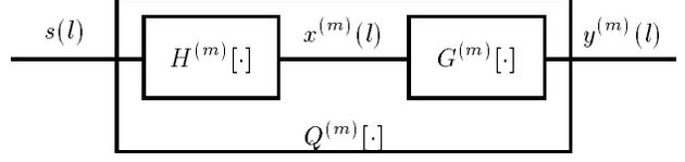
Figure 2: Channel  $m$  with linearizing equalizer.
