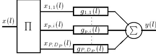
Figure 1: Volterra filter in Diagonal Coordinate System
