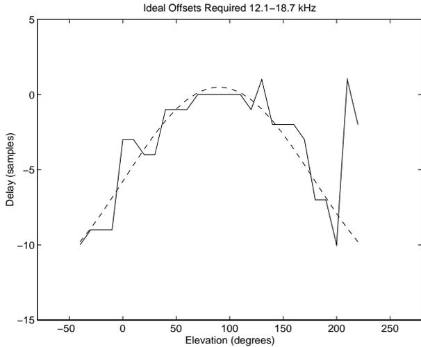
Figure 6: Sinusoid fitted to the pattern of delay vs angle, for the frequency band 12.1-18.7 kHz.
