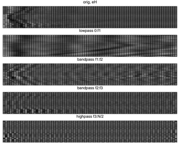
Figure 2: Image presentation of data. Time is from left to right, 80 samples at 44100 Hz sampling rate. Each of the 27 rows corresponds to an angle of elevation, from -40 deg. to 220 deg. at 10 deg. intervals. Top image: original data; lower images are low-pass, and then progressively higher frequency bands.
