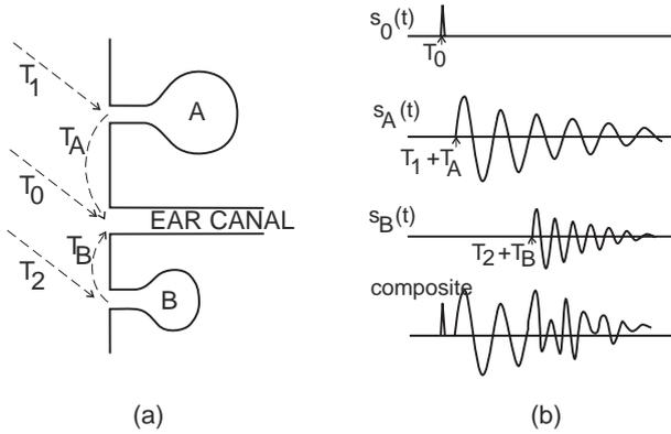
Figure 3: Principle of bottle model. (a) Simple geometric model with two “bottles” (resonators), A and B, showing how signals are received at the ear canal with delays  $T_0$ ,  $T_1 + T_A$  and  $T_2 + T_B$ , dependent on the direction of arrival. (b) Contributions  $s_0(t)$ ,  $s_A(t)$ , and  $s_B(t)$  and their sum at the ear canal.
