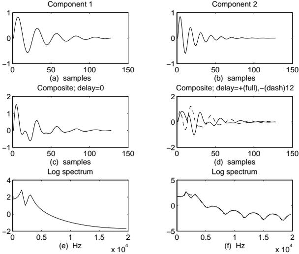
Figure 1: Effects of damped cosines added with delays. (a), (b) pole responses; (c) superimposed, no delay; (d) superimposed with +12 (full line) and -12 (dashed) sample delays; (e) logarithmic magnitude of transfer function with no delay; (f) logarithmic magnitude of transfer function of composite with relative delays. the full and the dashed lines correspond between (d) and (f).
