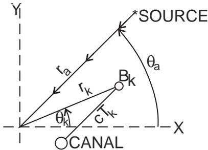
Figure 4: Geometry for  $k$ th coplanar bottle  $B_k$  and source.
