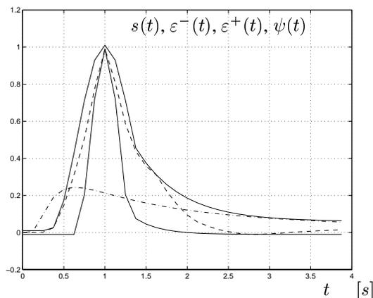
Figure 2: Input signal  $s$  (dash-dotted line), specified output envelope  $\varepsilon$  (solid line) and resulting noiseless output signal  $\psi$  (dashed line).
