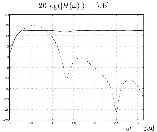
Figure 3: Resulting frequency response of equalizer for an  $L_\infty$ -design (solid line), and an  $L_2$ -design (dashed line).
