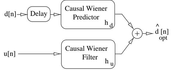
Figure 3: Optimal Estimator
