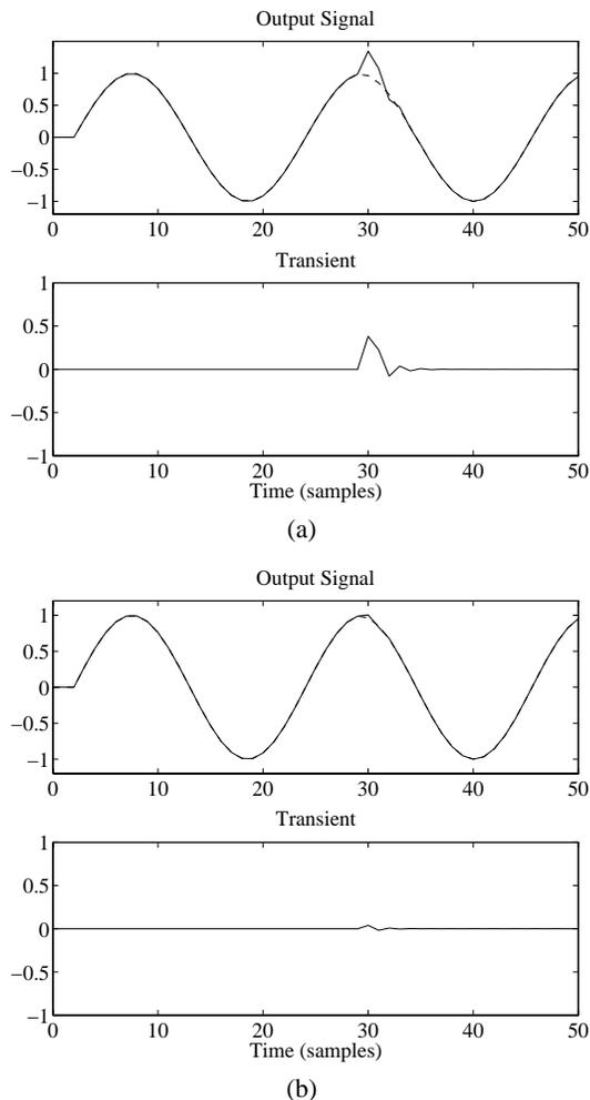
**Figure 3.** The output signal waveform of a second-order allpass filter (DF II structure) when the coefficients are changed at time index  $n = 30$  (a) with no transient elimination and (b) with the proposed transient suppressor with  $N_a = 4$ . The difference (transient) of the actual and ideal (dashed line) output signals is also displayed.
