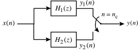
**Figure 1.** The output-switching method.
