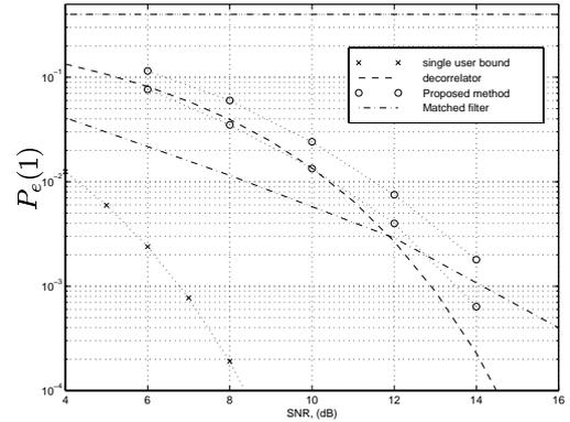
Figure 1: Probability of bit-error vs. SNR for proposed method using a short (20 bits) training sequence, for a near-far ratio of 0 (lower) and 10 dB (upper).
