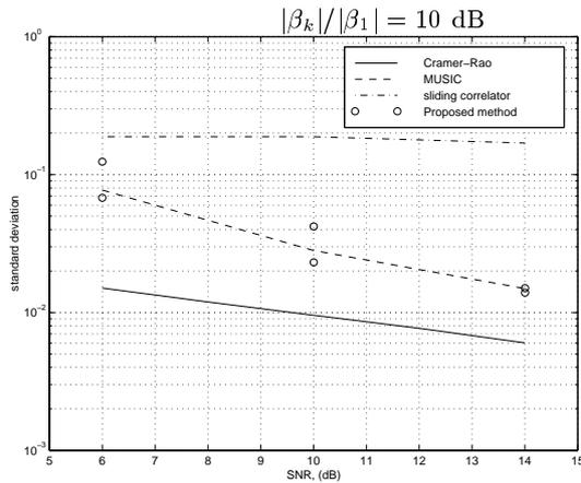
Figure 4: Same as figure (3) with a near-far ratio of 10 dB.
