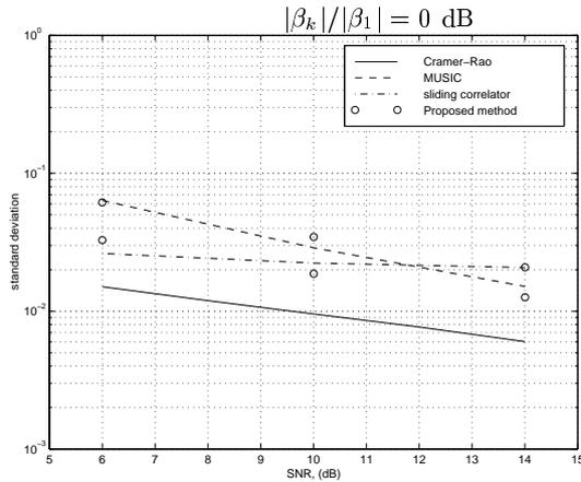
Figure 3: Standard deviation of estimation error in  $\hat{\tau}_1$  for a near-far ratio of 0 dB, for short (upper) and long (lower) training sequence, respectively
