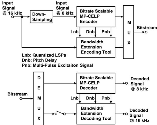
Figure 1. A block diagram of the proposed coder with both bitrate and bandwidth scalabilities.
