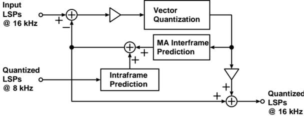
Figure 4. A block diagram of LSP quantizer.
