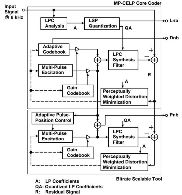
Figure 2. Bitrate scalable MP-CELP coder.
