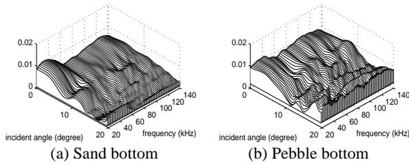
Fig. 5 Estimated backscattering coefficient as a function of frequency and incident angle
