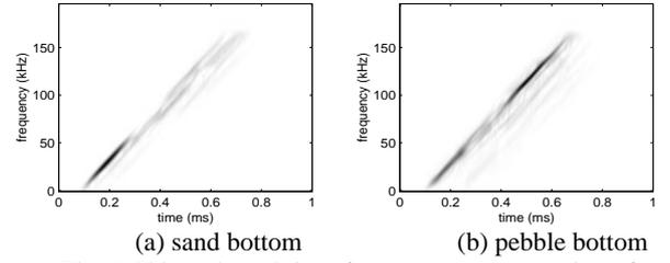
Fig. 3 Chirp adapted time-frequency representation of bottom echoes
