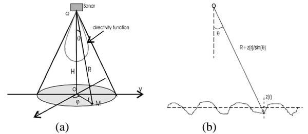
Fig 1. (a) Echo collection configuration., (b) Description of local roughness
