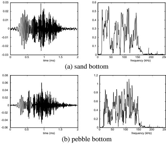
Fig. 2 deconvolved signals and their spectrum
