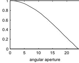
Fig.4 The directivity function of our used sonar
