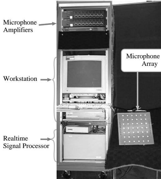
Figure 5: Realtime Signal-Processing System (S-RTP2000) and a Workstation.
