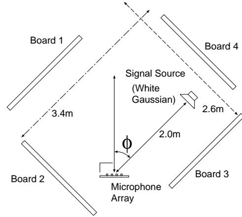
Figure 6: Experimental Set-up.
