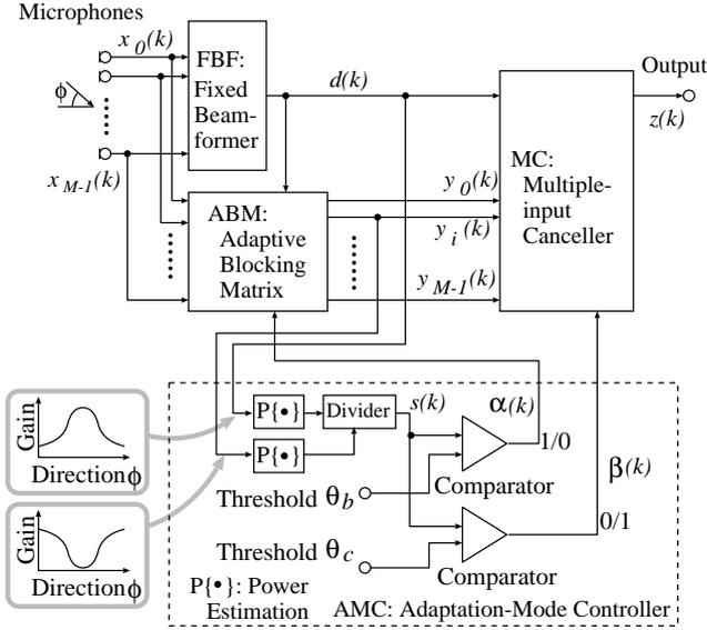
Figure 1: Structure of RAMA-ABM with AMC based on SNR estimate.
