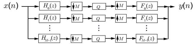
Figure 1.  $M$ -channel filter bank.
