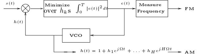
Figure 1: Block diagram for the AM-FM demodulator; AM in Figure corresponds to the traditional envelope of  $1/h(t)$  (i.e.  $1/|h(t)|$ ) while FM denotes the positive Instantaneous Frequency of  $s(t)$ 's All-Phase component.
