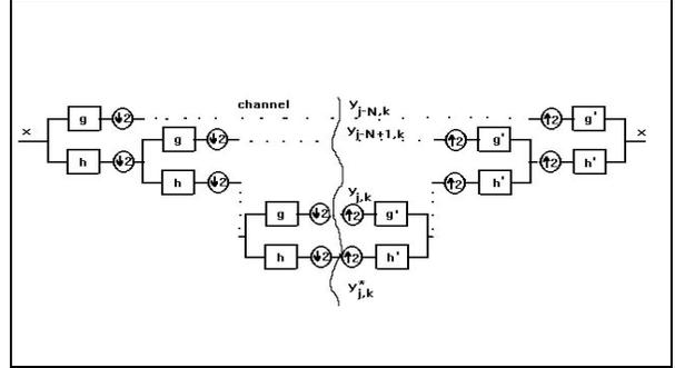
**Figure 1.** Iterated two-channel filterbank for multi-resolution analysis
