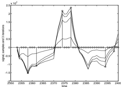
**Figure 6.** Detail of reconstruction of the signal in Fig.4: signal, remaining samples in this interval, iterations in the on-line reconstruction, illustrating convergence.
