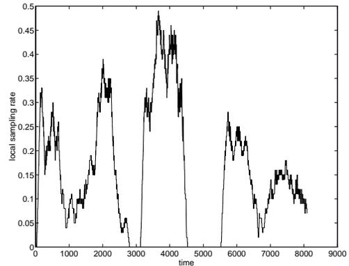
**Figure 7.** Instantaneous sampling rate for the signal in Fig. 4, obtained by averaging the number of remaining samples over 100 consecutive values of the signal, an indication of the instantaneous frequency.
