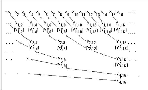
**Figure 3.** Adaptive sampling algorithm after a 4 iteration-level analysis
