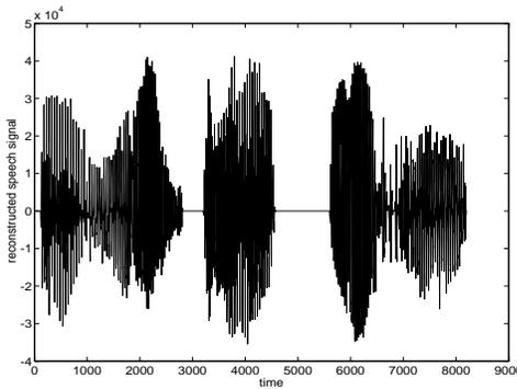
**Figure 5.** Reconstructed signal, out of 1289 remaining values after adaptive sampling using rel. (17) iterated 9 times
