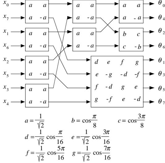
Fig. 3 8-point DCT.
