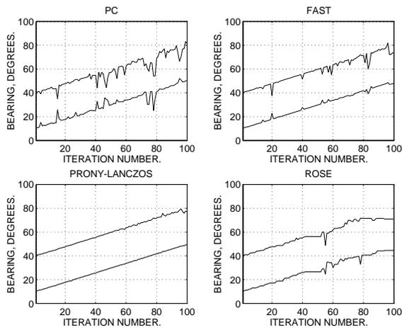
Figure 3: Bearings from PC, Prony-Lanczos, FAST and ROSE.
