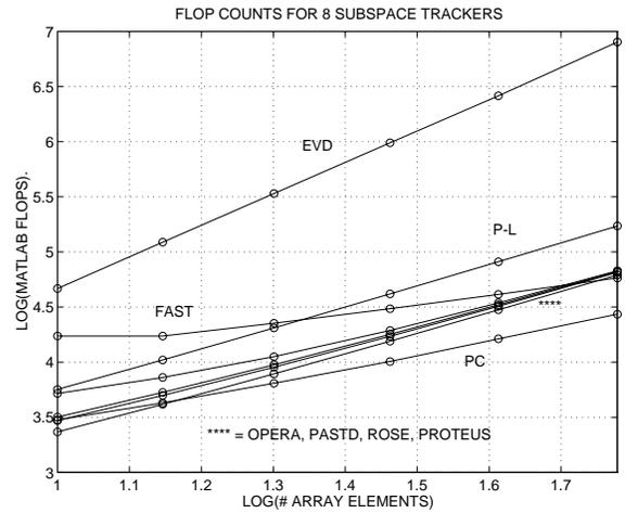
Figure 1: Flop Count vs Array Size for 8 Subspace Trackers.
