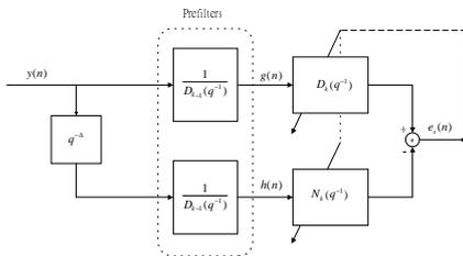
Figure 2: SMM using ALE for notch filter identification.
