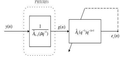
Figure 5: Equivalent block diagram of SMM-ANF for off-line frequency estimation.
