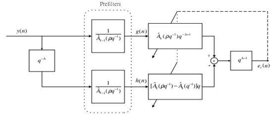
Figure 3: Block diagram using SMM in an ALE structure. It is unrealizable due to the advance operator for  $\Delta > 1$ .
