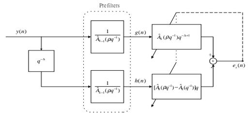
Figure 4: Block diagram of SMM-ANF
