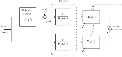
Figure 1: Block diagram of SMM for system identification.
