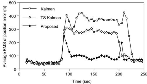
Figure 4: Average RMS position errors versus time
