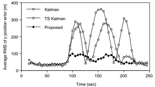
Figure 6: Average RMS y-axis position errors versus time
